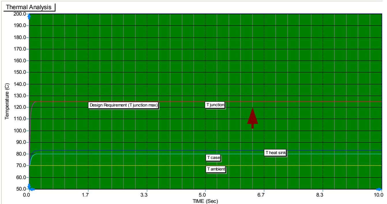
Eureka, everything meets the design requirement. Only one small problem, I can't use convection cooling, the thermal resistance isn't low enough. Well maybe I can use forced air. After referring to the thermal curve - illustration 1. I determine even at a 1000ft/min I can only realize a thermal resistance of 0.8 °C/W; not nearly enough. From my past analysis, I require 0.36°C/W. At this point, I think, I'm in deep stuff.
